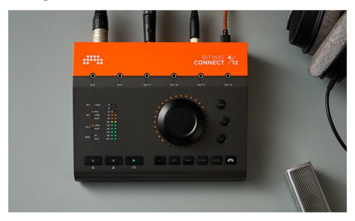
Bitwig announces its first hardware product: Bitwig Connect 4/12. It's more than an audio interface – it's a class-compliant, 4-in/12-out CV and MIDI-enabled audio interface with monitor- and DAW-control functionalities and a unique Bitwig Mode. As a bridge between software and external gear, Bitwig Connect is the perfect device to mark our debut into hardware.
