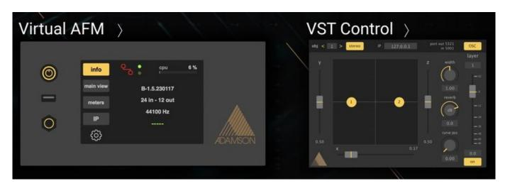
The Virtual Adamson Fletcher Machine (vAFM) connects with the Adamson Fletcher Machine (AFM) Remote software, giving users the Fletcher Machine experience without the requirement of a dedicated hardware engine (Stage or Traveler). Instead, the user employs the audio I/O available on the computer the vAFM is installed on.
