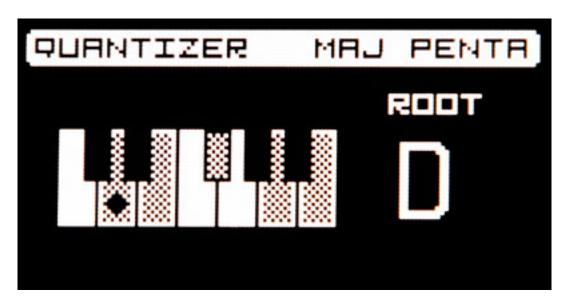
SHIFT+SCALE opens the quantisation-dialog where the user can either select a predefined scale, create a new scale and change the root note.
