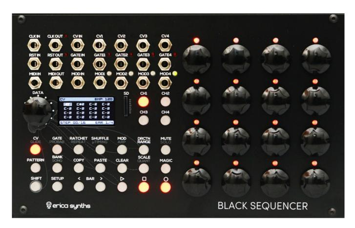
Power consumption tops out at 114mA at +12V and 24mA at -12V. This is quite moderate compared to other sequencer modules. +5V is not required.
