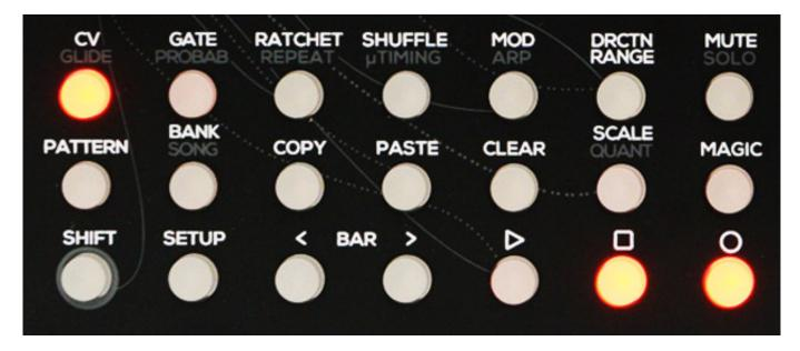
The lower row offers access to relevant system functions such as configuration, starting, stopping and saving the current configuration. Whenever a pattern has been changed the record-key denoted by a circle blinks. By the way, all buttons are illuminated by red LED's as indicators. So much for the basic handling of the sequencer.
