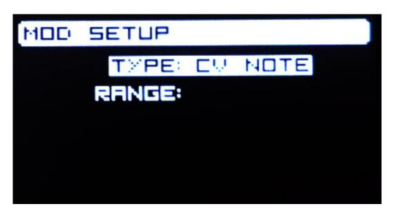
Let's have a look at the modulation output that has a multitude of uses. Pressing SETUP+MODE accesses the configuration dialog.
