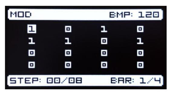
Another very interesting modulation mode is the trigger mode. Every step features a trigger impulse configured (turned on / off) by pressing on the corresponding encoder, enabling a tighter integration with drum and percussion modules. The flexibility is slightly hampered by the limited range of lock divisors but sufficient for
