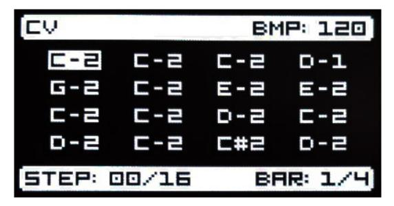
The CV key switches the Black Sequencer into CV mode. The display now shows the notes assigned to the current 16-step window. Turning one of the 16 rotary encoders directly modifies the respective step, which is emphasised by the appearance of a pop-up with the current value. Like I mentioned before this pop-up can be deactivated in the system settings.
