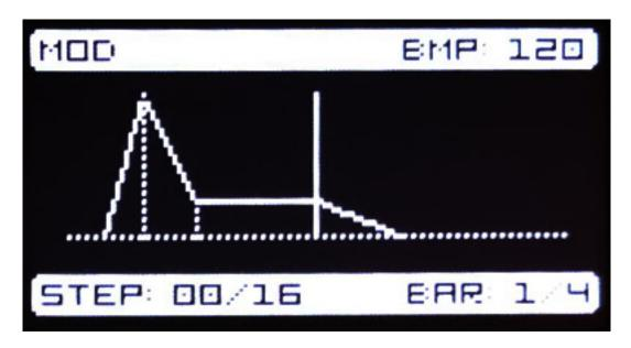
It is possible to output a defined voltage or a voltage corresponding to a note. There are also modes to output AD, ASR or ADSR envelopes.
