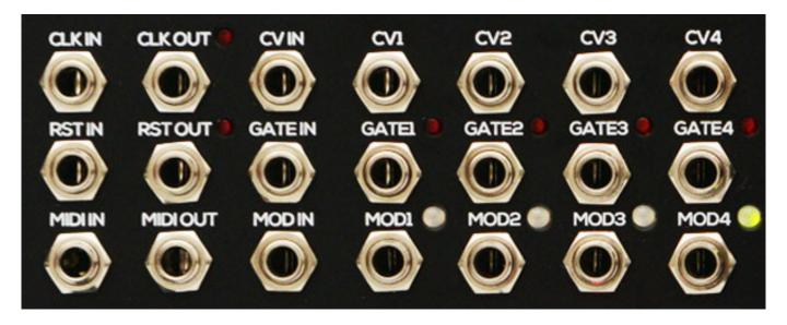
Let's have a look at the connections first. On the right hand side you will find the outputs for CV, gate and modulation voltages for the four tracks. To the left there is one input each for CV, gate and modulation. The Black Sequencer also sports inputs for clock, reset, MIDI in- and output, all as 1/4" (3,5mm) TS sockets.
