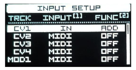
The Black Sequencer supports clock and reset in- and outputs and MIDI Clock. Since firmware 1.01 it is possible to use the VC- and MIDI-Input for example for key-transposition of a track. Thge assignment and function can be configure in the Input-Setup dialog. A real MIDI keyboard live recording with quantization will be available with the next firmware.
