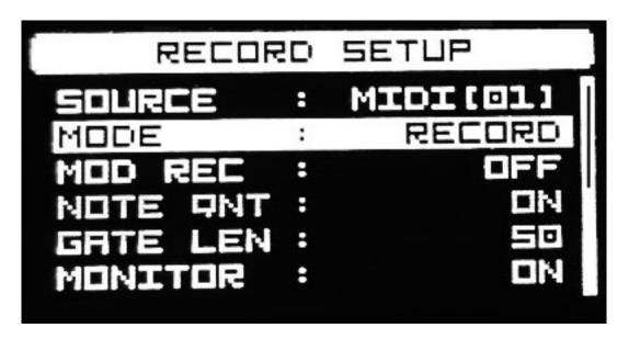
The firmware 1.02 offering also a recording via a connected MIDI or CV-Keyboard. There are tweo real time and two offline recording modes. OVERDUB records realtime and add notes and RECORDING overwrites existing notes. If the record function is armed the recording starting by pressing a key on the keyboard. In both mode a visual precounter can be activated via the POP-UP parameter in the
