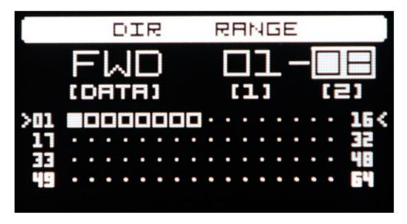
DRCTN RANGE accesses a dialog that controls the playback-direction of the current pattern: forwards, backwards, ping-pong and random. Also the playback range (start and end point) can be set by pressing one of the 16 encoders.
