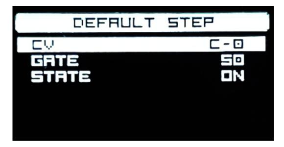
There is also a dialog to configure the standard settings of a step: note and gate length.
