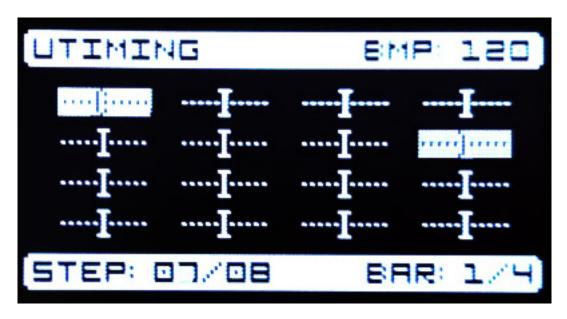
UTIMING (Microtiming) offers even finer grained control for every individual gate step. And then there is the track related MAGIC function that causes all or specific
