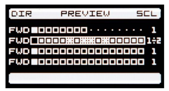
With the key combination SHIFT + DRCTN RANGE a 16 step overview of all four tracks appear including playback mode and clock divider/multiplier.
