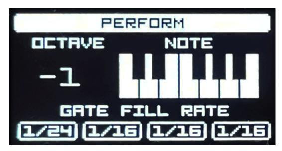
In the 1.0 release there is a perform dialog available for transposing by the first 12 encoders and rolls can be filled by pressing the encoders 13 until 16. The roll rate can ajusted by these four encoders.
