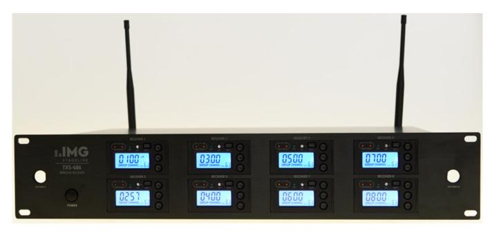
From the wide range of receivers available, we would like to show you the top model TXS-686 which features eight receiver channels and is accommodated in a 19" housing with 2 RS. The receiver is equipped with a diversity receiver and thus provided with two antenna jacks (BNC). The device is supplied with respective antennas.
