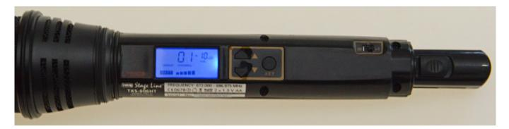
A small sliding switch at the bottom of the handle allows you to change the transmitting power between 2.5mW and 25mw EIRP. For practical reasons, this switch is only accessible when the cover of the hand-held device has been unscrewed. The large sliding switch also allows you to switch-off the hand-held microphone when the cover is screwed on.
