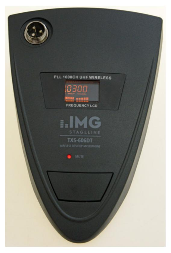
The base features an integrated LED at the bottom for indicating the mute status as well as a display giving information on group, channel and battery status. The desktop transmitter is operated via two batteries AA size which allow an operating time of more than eight hours. Pressing the button on the top of the base allows you
