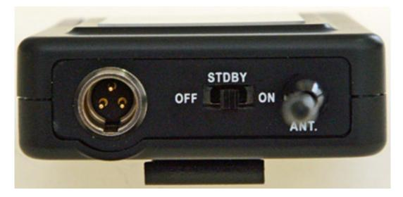
A mini XLR jack (unbalanced connection) is located at the top of the device (see photo above) for connecting an electret microphone, e.g. headset microphone HSE-80 from IMG STAGELINE. A supply voltage for electret microphones is available at the jack. The transmitter can be switched on (ON), off (OFF) or be switched to standby (STDBY) via a 3-step sliding switch.
