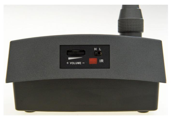
You can set the microphone sensitivity on the rear panel of the desktop transmitter and use a sliding switch to select the transmitting power between 2.5mW and 25mW EIRP.
