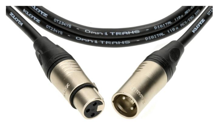
KLOTZ AIS now supplies the new PD7 Pro Digital series with the high-quality OT234YS low loss cable for AES/EBU and DMX signals. The connectors available are either the XLR 3p. and XLR 5p. plugs by KLOTZ or Neutrik. The double shielded OT234YS has a massive conductor cross-section of 0.34 mm<sup>2</sup> (AWG 22/7) and is ideal for professional applications thanks to the durable PVC jacket.
