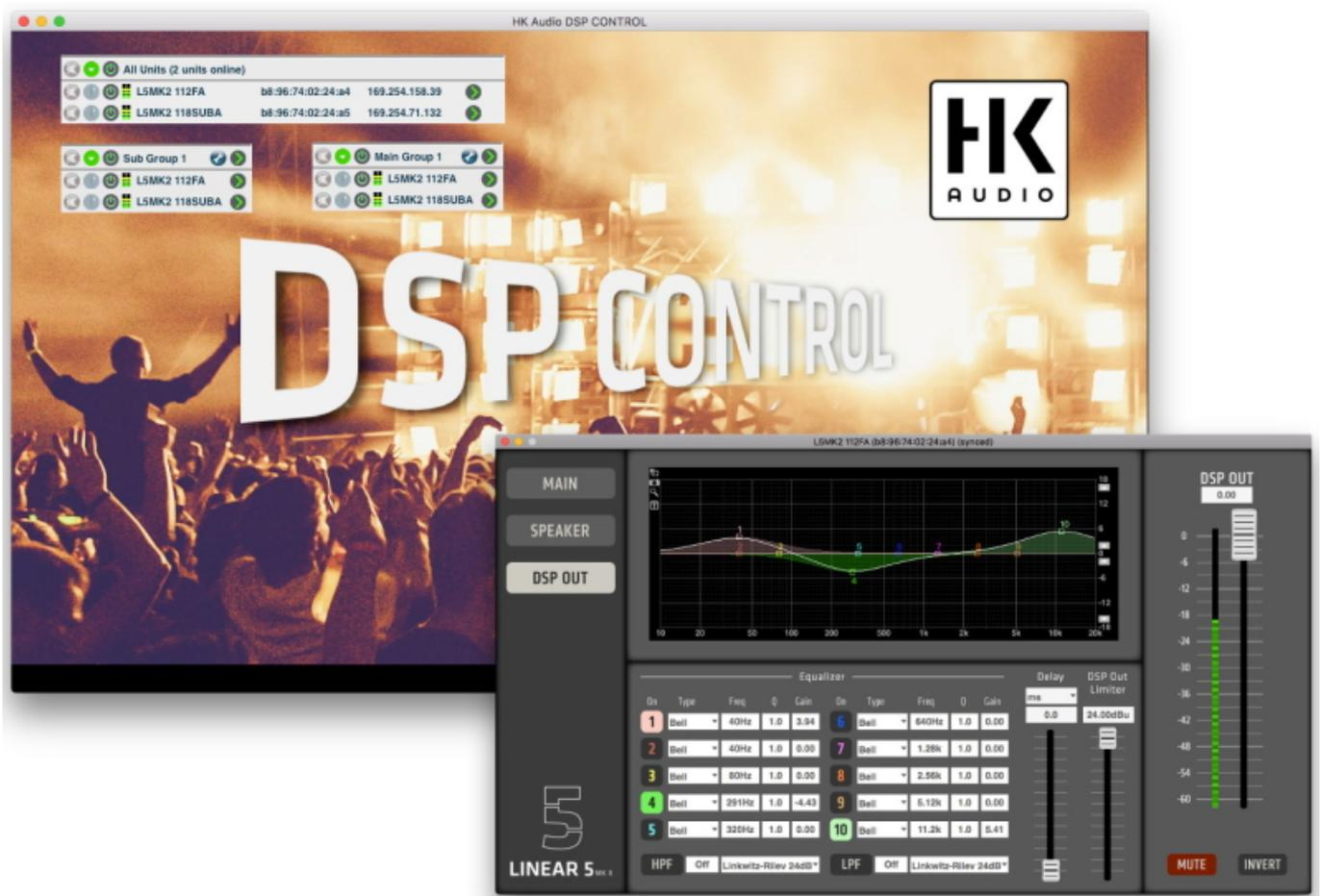
HK Audio DSP CONTROL is a comprehensive and easy-to-use software for Mac and PC for precise sound tuning, firmware updates and remote control of the DSP parameters of all network-enabled HK Audio speakers of the ELEMENTS D, LINEAR 5 MK II, LINEAR 7 and LINEAR 9 series.
