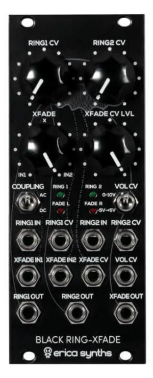
The Erica Synths Black Ring-Xfade is an extremely versatile module for sound shaping. It consists of two unconventional ringmodulators/waveshapers, a crossfader that works both for audio and CV and a VCA. Unlike conventional ringmodulator that works only with a signal present on both signal and carrier inputs, the Black Ring-Xfade passes through the signal without alteration, if no
