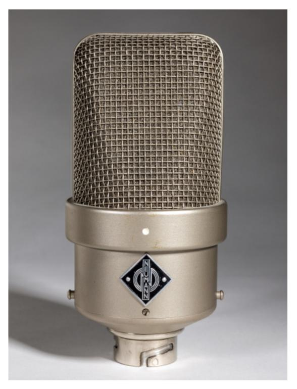
The Neumann M 50, which was introduced in 1950, was instrumental in the development of the Decca tree recording technique. Its open-mesh head basket houses a small-diaphragm capsule flush-mounted in a small sphere, and its unique acoustic properties are ideally suited to orchestral recordings.
