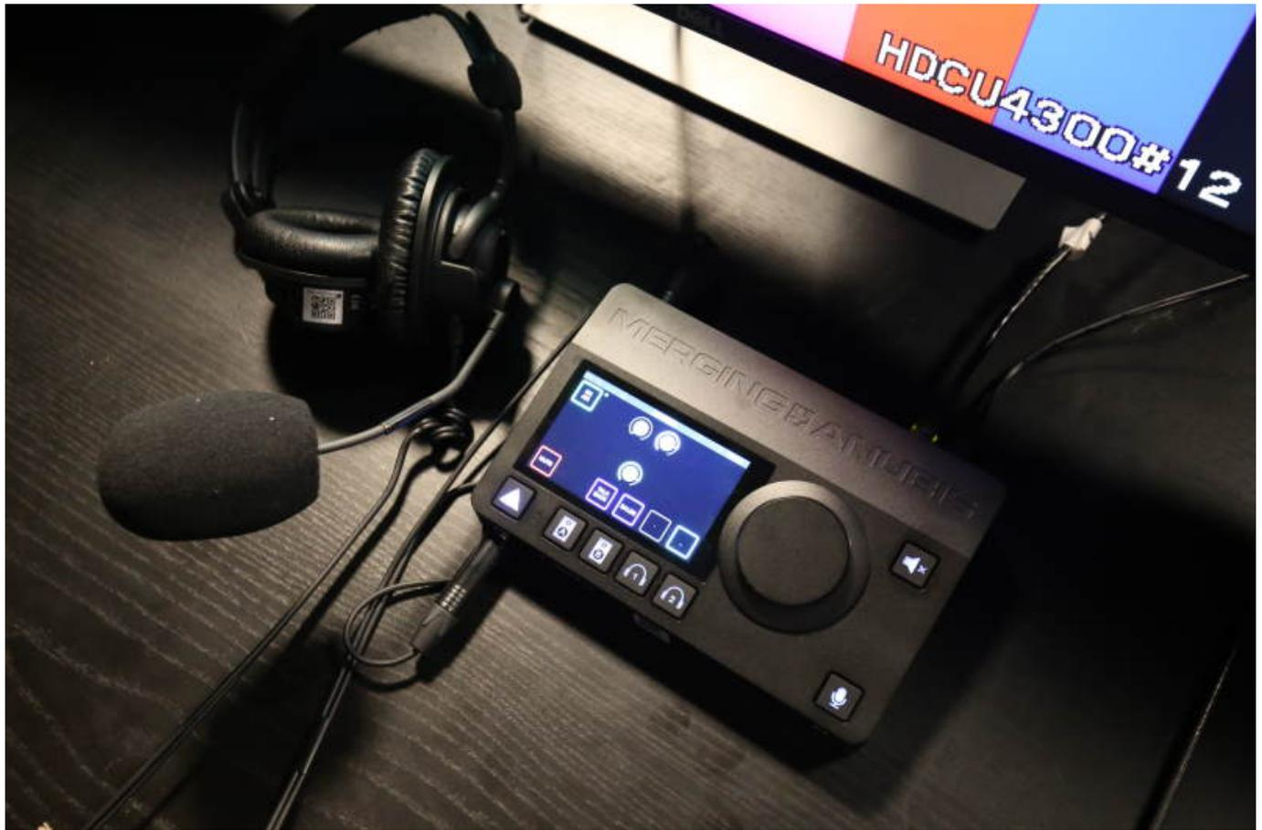
When operating the unit, both commentators can control their access to the On-Air output, can Mute their microphone (Cough Cut) and can talk to up to 4 available Talkback outputs. All these controls can be configured to be hidden, locked, latch/press-release, renamed, to offer an as safe and easy to operate experience. Various monitoring options are also available to customize the monitoring behavior when operating these controls.
