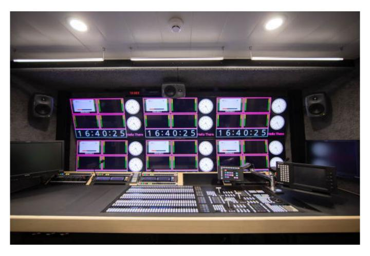
Each truck offers 36 vm\_dmv heads delivered by V\_matrix C100 blades for multiviewing purposes. Overarching control and orchestration is managed by Lawo's VSM IP control system.
